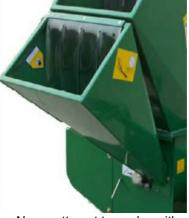
The lower chute is for longer and/or thicker pieces of yard waste. Depending on your model, you may cut up to a 3" x 5" in piece of wood.
