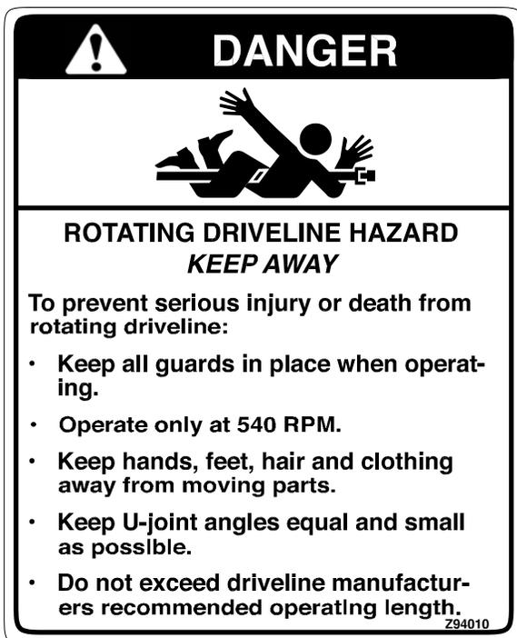
REMEMBER - If safety signs have been damaged, removed, become illegible or parts replaced without safety signs, new signs must be applied. New safety signs are available from your authorized dealer.
