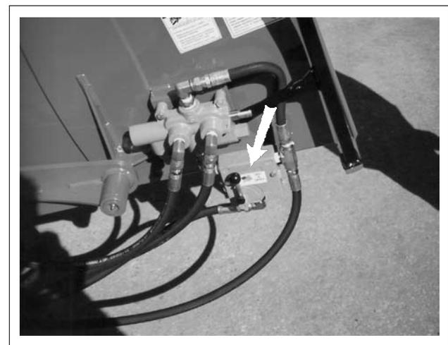
Fig. 22 FLOW CONTROL VALVE
